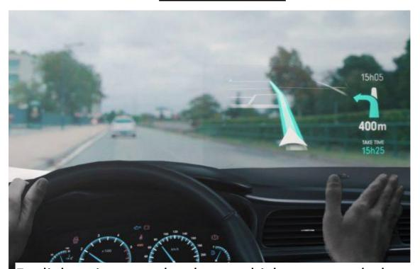
Eyelights is a technology which uses a holograph instead of a real screen to display information like maps, vital stats related to the car, speed etc. This allows you to keep an eye on the road even while interacting with the system. Further, since there is no physical screen, you can simply wave your hand in the air to control the system which makes it super easy.
